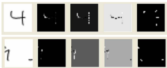
Figure 4. The left most images in each row are the candidate and context images rendered at 29x29 pixels. The remainder of each row shows various feature images computed from these principle images. From left to right: stroke curvature, stroke normal X, stroke normal Y, and endpoints.
